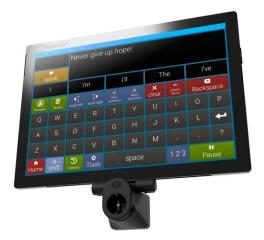
The new eye gaze camera from Eyegaze Inc. Features include dual eye tracking, tolerates increased head movement (as compared to the Edge), smaller more durable design. You can complete live calibration adjustments – by clicking and dragging to locations on the screen where the person can access.
